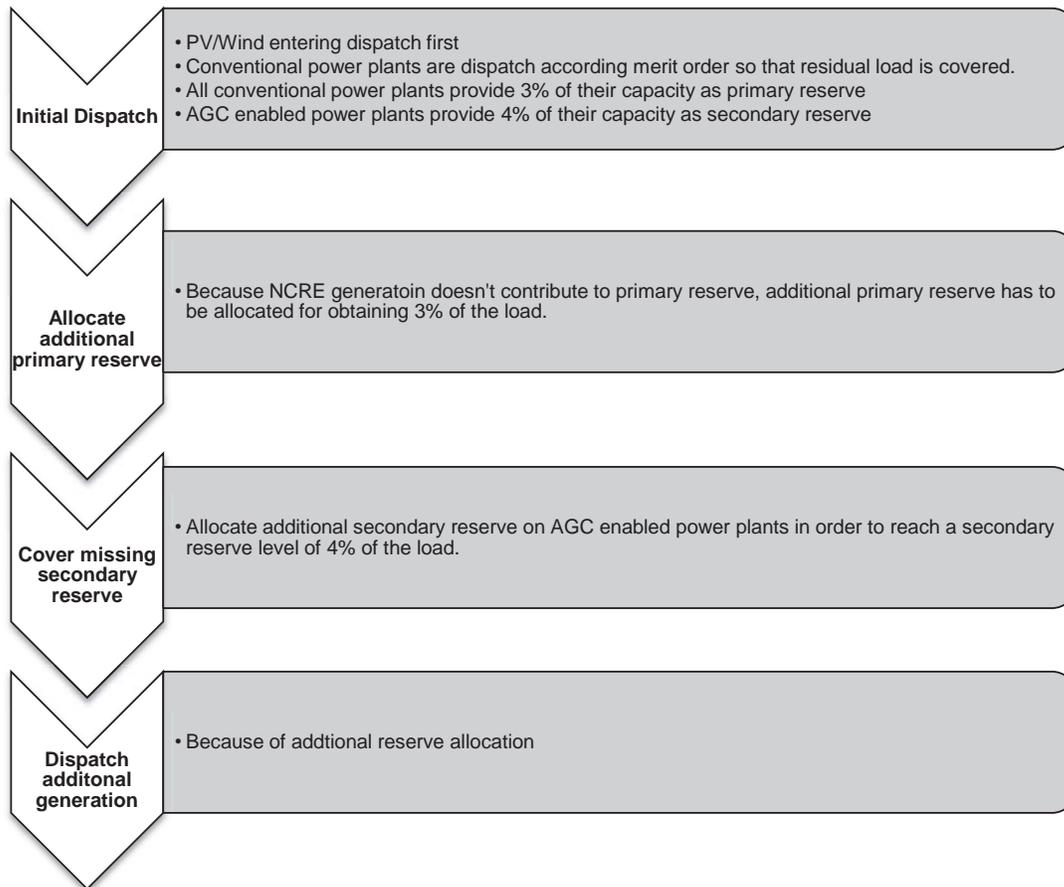
Figure 7: Algorithm for calculating the generator dispatch
