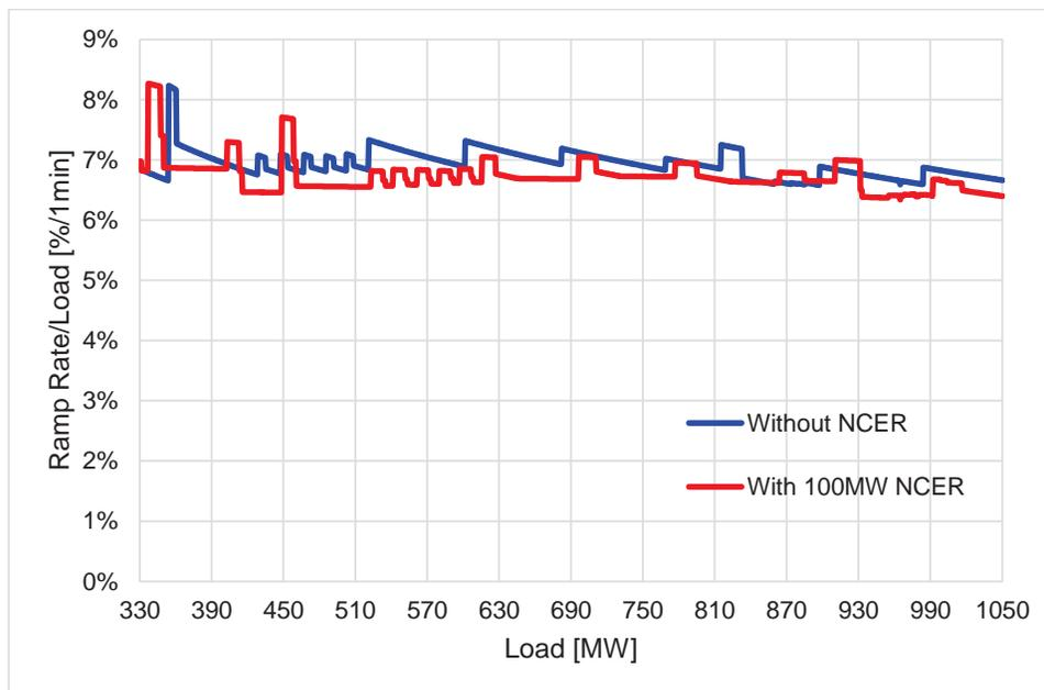
Figure 13- 1min Ramping capabilities of Spinning Reserve during dry season
