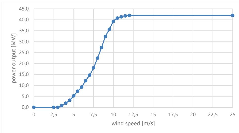
Figure 4: Power Curve of representative wind farm
