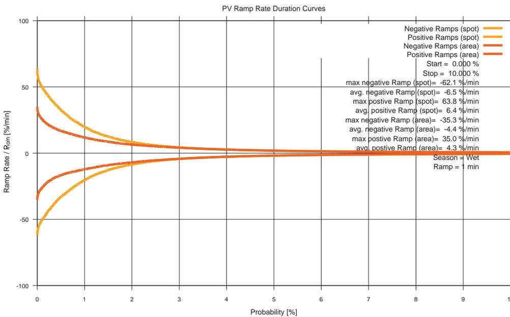
Figure 3 – Cumulative probability curve of ramp rates of PV generation with diversity (orange) and without diversity (red)
