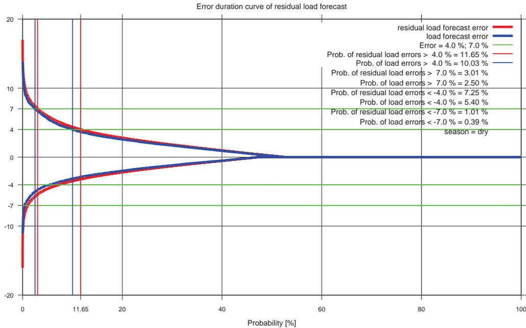
Figure 9 – Day-ahead prediction error of Residual Load and Actual Load during dry season
