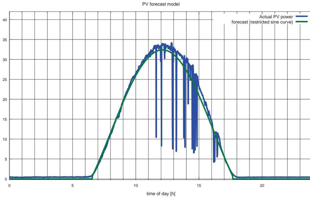
Figure 5: PV Prediction and actual PV generation of a representative day
