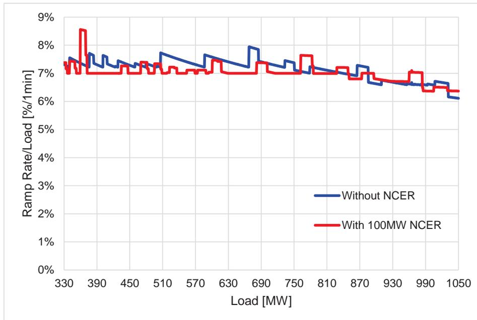
Figure 14 – 1min Ramping capabilities of Spinning Reserve during wet season
