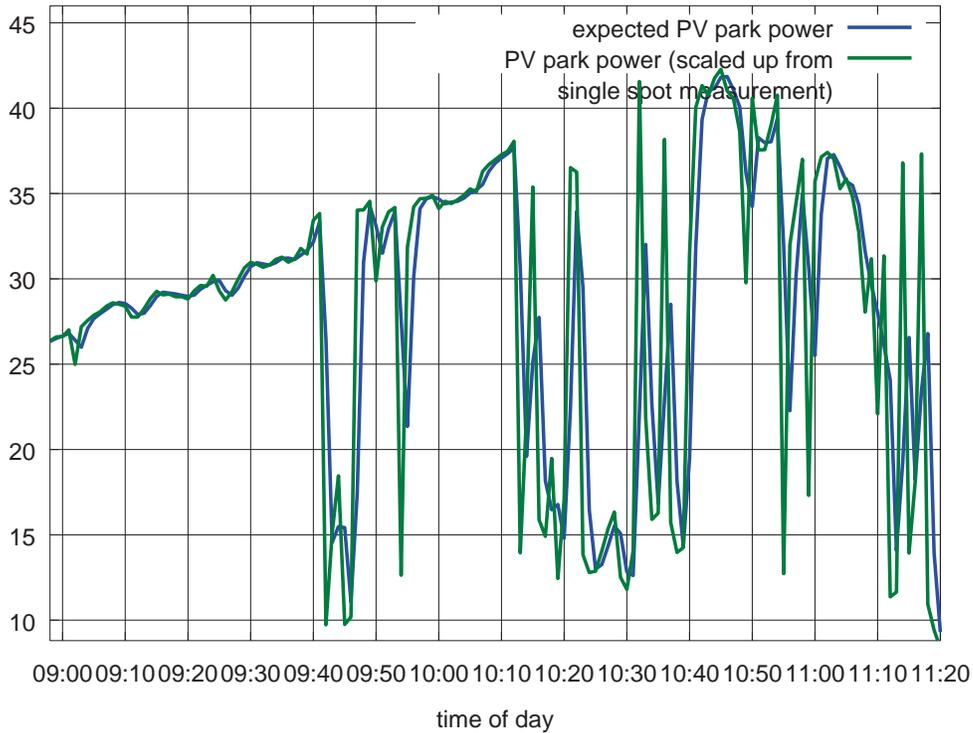
Figure 2 - PV time series with cloud simulation
