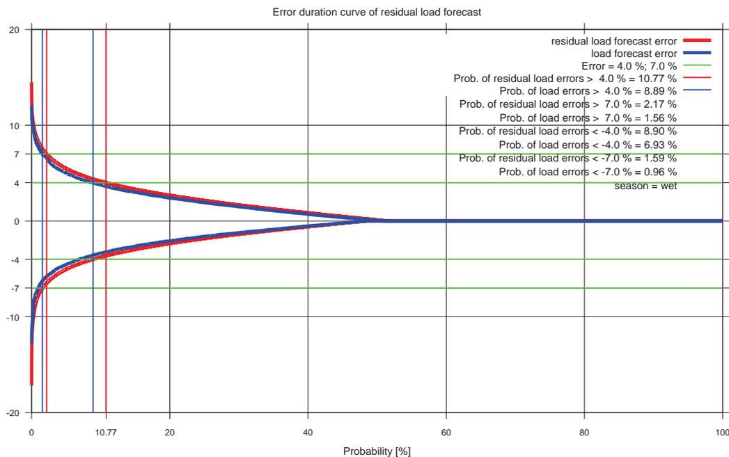
Figure 10 - Day-ahead prediction error of Residual Load and Actual Load during wet season
