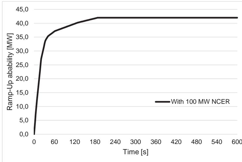
Figure 8 - Ramping Capability of AGC controlled power plants (Example: Wet Season, Load 1050 MW)
