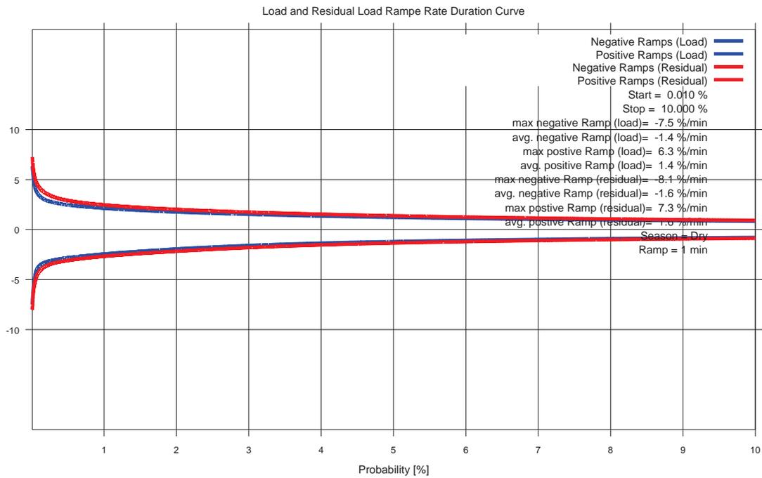
Figure 11- Ramp rates of Residual Load and Actual Load during dry season
