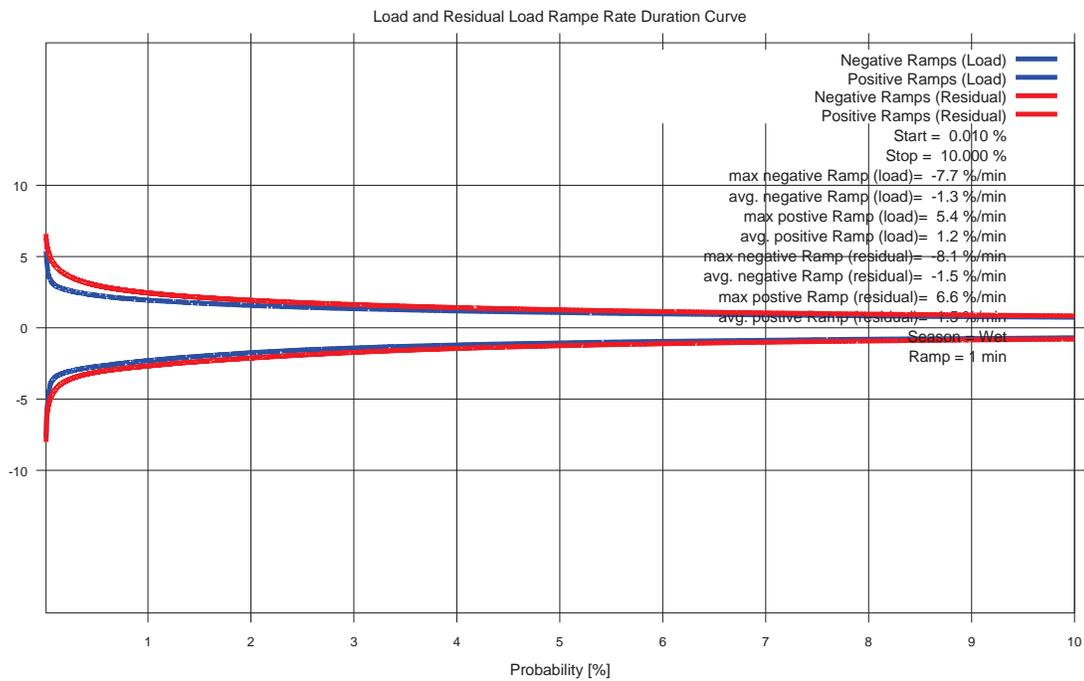
Figure 12- Ramp rates of Residual Load and Actual Load during wet season
